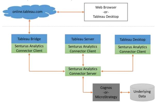
In the second and third cases, it is not necessary to install Analytics Connector client on Tableau Desktop that access the published data sources (TDS) through Tableau Server or Tableau online.
