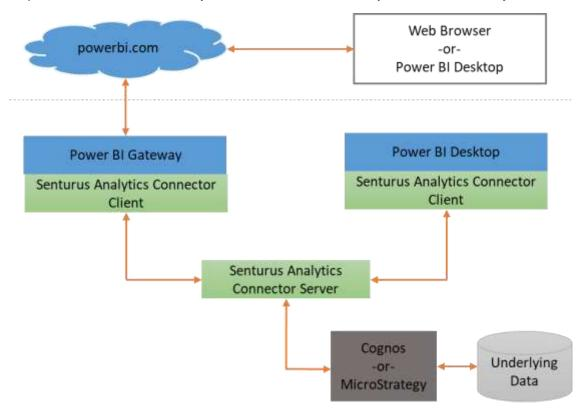
It is not necessary to install Analytics Connector on the local machines where Power BI Desktop is used to access the published data sources (Power BI datasets) through the Power BI service or for users who only view or modify visualizations on the Power BI service using a web browser.
