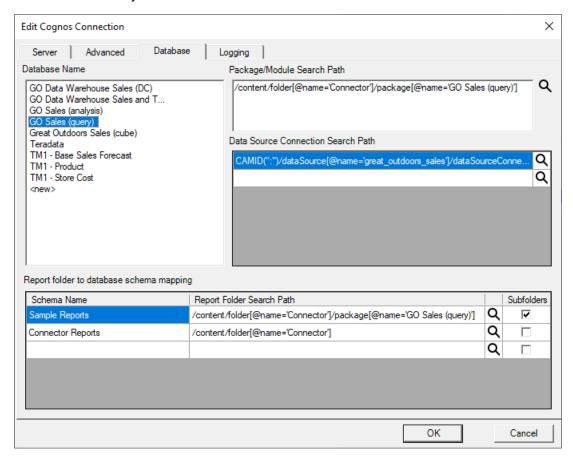
To edit an existing database, select the database name in the "*Database name*" list, and edit associated properties. To change the database name, double click on its name.
