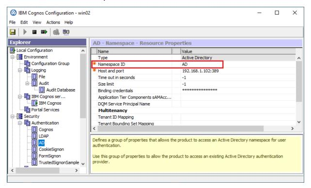
Alternatively, the Namespace ID can be found from the Cognos Adminitration console. Select the **Security** tab, click the **Properties** button ( ) next to the namespace, and click the link to view the Namespace ID ( View the search path, ID and URL ). The Namespace ID will be displayed in the **Search path** property. For example, **AD** is the Namespace ID you would use from the below
