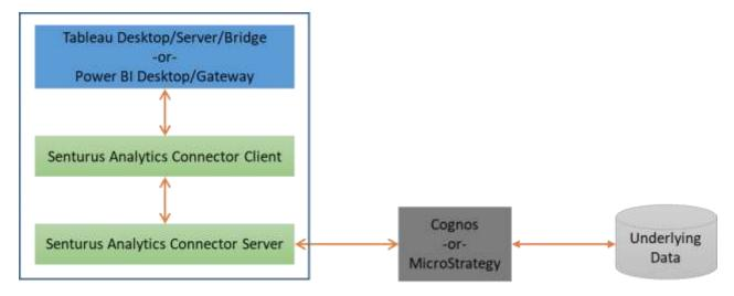
To install in this mode, follow Server Installation, Data Source Configuration and Service Configuration to install and configure Analytics Connector server on a computer.
