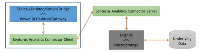
To install in this mode, follow Server Installation, Data Source Configuration and Service Configuration to install and configure Analytics Connector server on a server, then follow Client Installation to install the ODBC client on each client computer.
